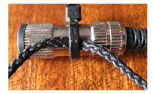
Attach the contact or the adapter with two cable ties as shown. One of the cable ties is tightened around the end pin.
