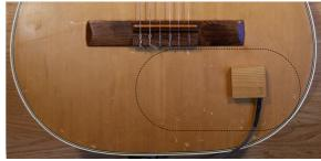
microphone in small moves. Attaching as shown on the image will be good for a start.
